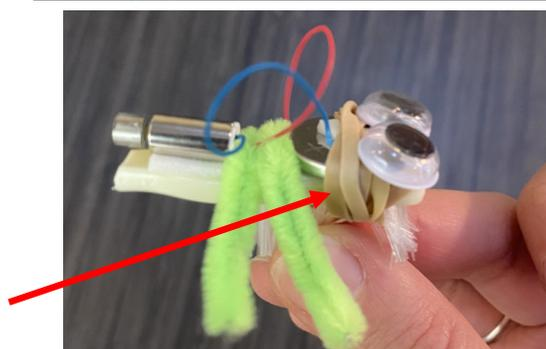
If the bristlebot does not turn on more pressure is needed in the connection between the battery and the wires. Try wrapping a rubber band around the battery to more firmly secure it in place.
